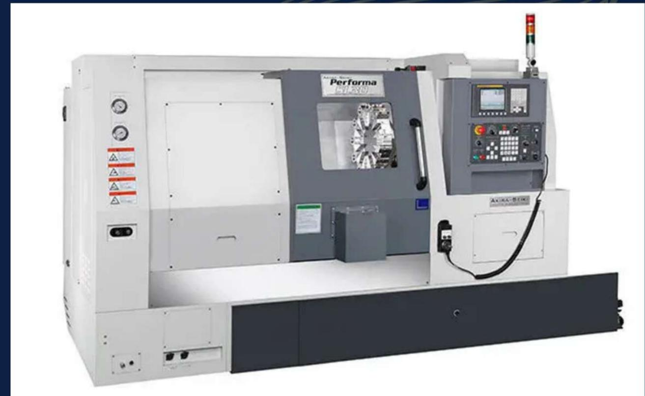
CENTRE DE TOURNAGE CNC A 3 AXES
